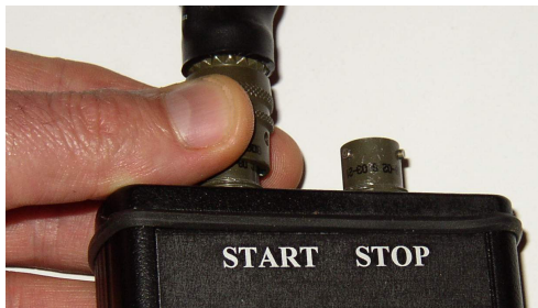
Figure 1. While connecting and disconnecting the transducers please touch the metal part only. This is very IMPORTANT! NEVER turn the plastic part of the connector.
