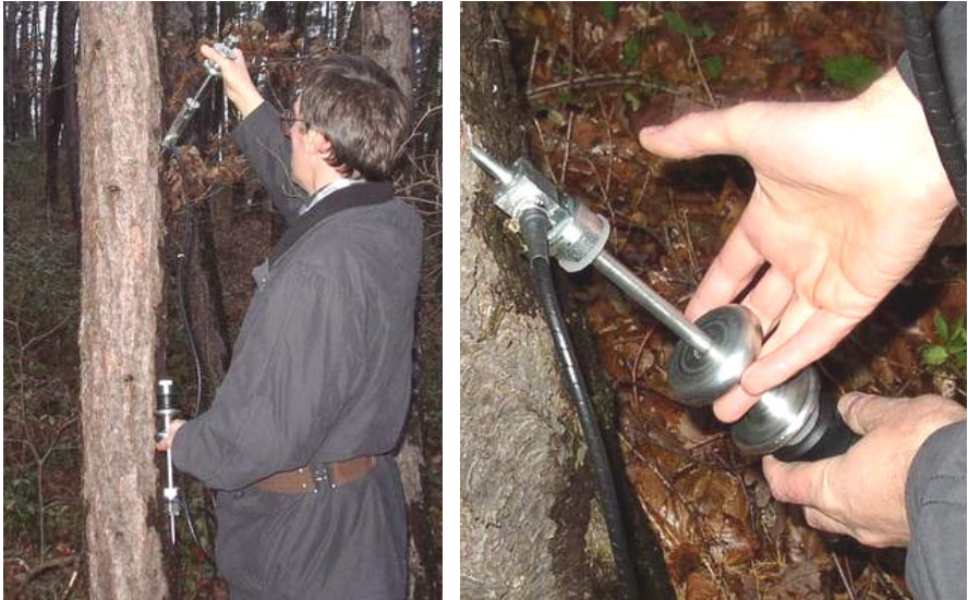
Figure 2. Driving the start (left) and stop (right) transducers into the tree using sliding hammer
