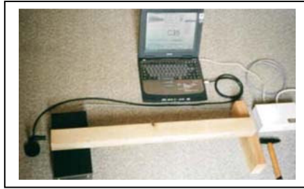
Fig. 5. The balance measures half timber load. This setup is demonstration only, recommended for long ( l > 2m ) lumber.
