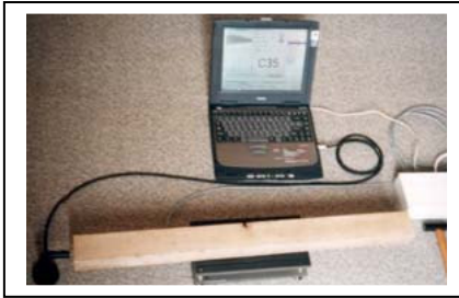
Fig. 4. The balance measures full timber load. Recommended setup for short (below 2m) lumber.
